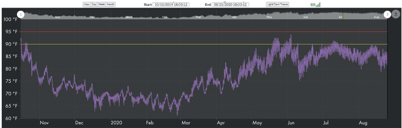
FIGURE 4 Seasonal temperature profile in the GeoGrid system showing the water temperature leaving the pumphouse.
